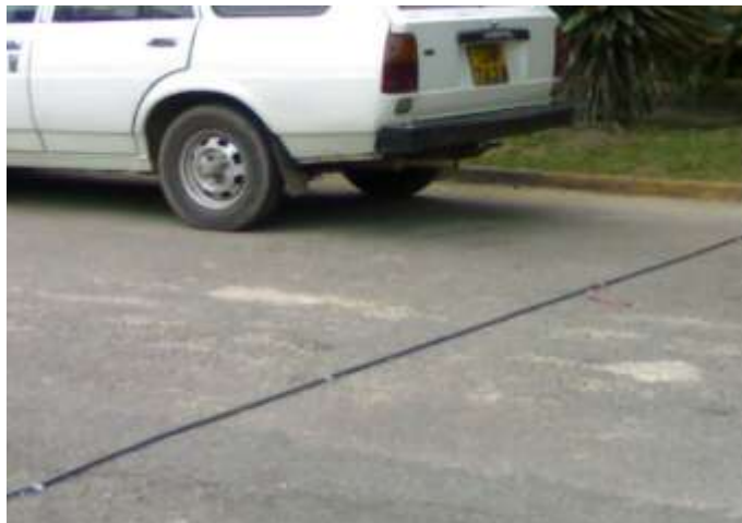
Fig 1.2 - Pneumatic rubber tube which connects to data logger
